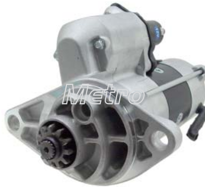
19201N Starter 12V, 3.0kw, CCW, 11T Battery Post M10
