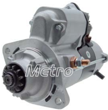
19120N Starter 12V, 2.7kw, CW, 11T Battery Post M10
